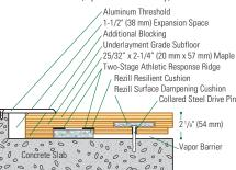
Slab Depression: 25/32" (20 mm) flooring - 21/8" (54 mm) • 33/32" (26 mm) flooring - 23/8" (60 mm)
