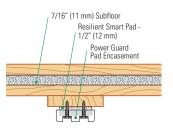
Slab Depression: Standard Profile Height 2 3/4" (70 mm)
