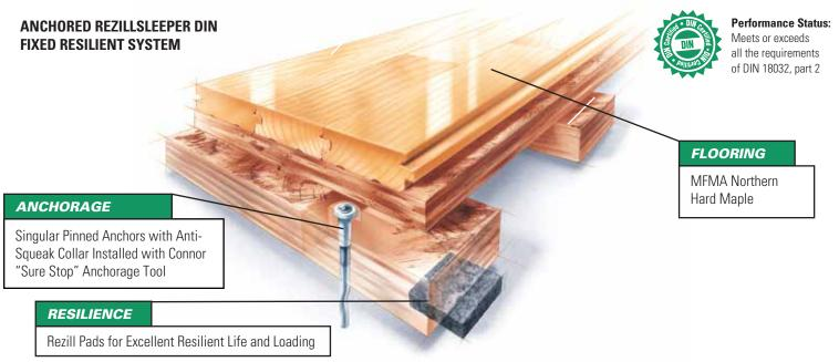
**Slab Depression:** 25/32" (20 mm) flooring - 2 5/8" (67 mm) • 33/32" (26 mm) flooring - 2 7/8" (73 mm)
