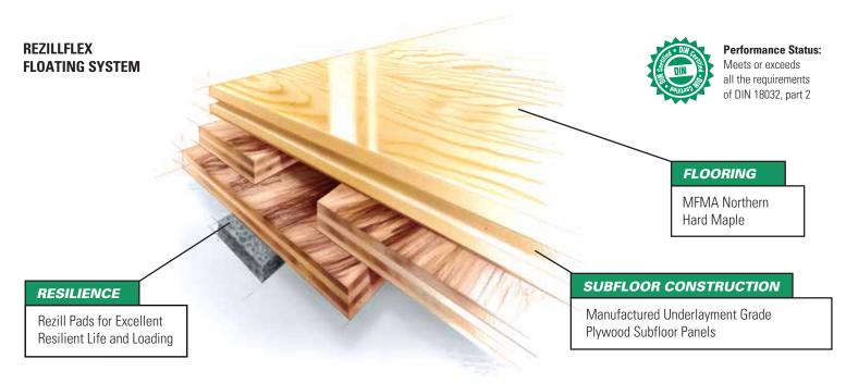
**Slab Depression:** 25/32" (20 mm) flooring - 2 1/8" (54 mm) • 33/32" (26 mm) flooring - 2 3/8" (60 mm)
