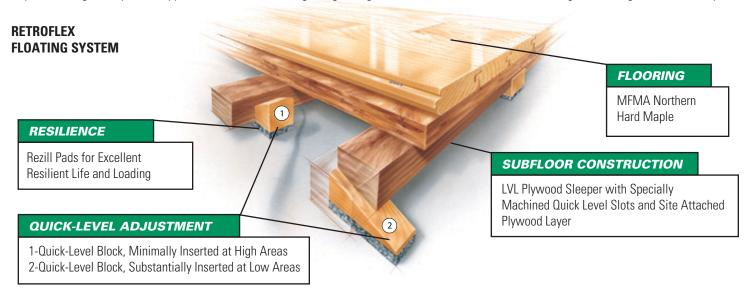
Slab Depression: 23/32" (18 mm) Plywood: 25/32" (20 mm) flooring - 3 1/4" (83 mm) Plus, 33/32" (26 mm) flooring - 3 1/2" (89 mm) Plus **15/32" (12 mm) plywood:** 25/32" (20 mm) flooring - 3" (76 mm) Plus, 33/32" (26 mm) flooring - 3 1/4" (83 mm) Plus
