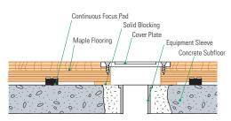
**Slab Depression:** 25/32" (20 mm) flooring – 13/4" (44 mm) • 33/32" (26 mm) flooring – 2" (51 mm)
