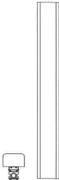
ANDREW - LNX-6515DS-A1M WEIGHT (WITHOUT MOUNTING HARDWARE): 43.7 LBS SIZE (HxWxD): 96.60x11.90x7.10 IN. MOUNTING HARDWARE P/N: DB380-3 & DB5063D RATED WIND VELOCITY: 149.8 MPH
