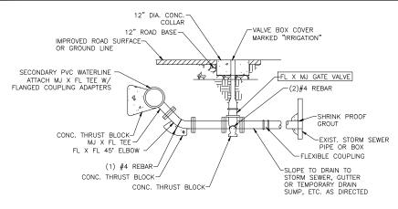
4" DRAIN VALVE DETAIL
