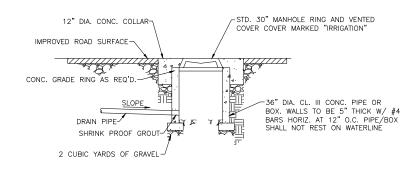
TEMPORARY GRAVEL DRAIN SUMP DETAIL
